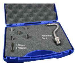
according to the European Standard EN 13284-1, includes a set of 5 nozzles and one gooseneck-curve for small tubes and openings (openings  $> G 2\frac{1}{2}$ ).
