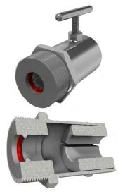
The lower half-pan is firmly screwed on while the upper pan is moved by a toggle. Shifting the suction tube works fast and easily through the toggle. The suction tube is not damaged by the half-pans even under strong loading. The half-pans are adapted to the required external Ø of the suction tube.
