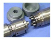
Connections between the parts, with seal material Nyhalit (up to 300°C)
